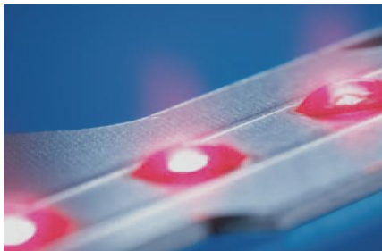
Chip On Board: The LED chip is directly bonded on to metal substrate for heat sinking
